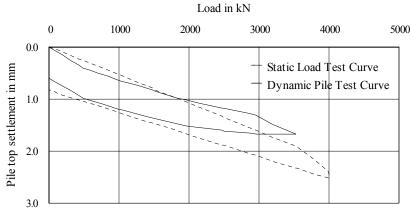
Figure 3 Pile No. P13-8 at National Park Flyover, Mumbai Static Test: 07/08/99; Dynamic Test 02/09/99
