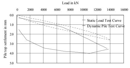
Figure 5 Initial Test Pile at JJ Urban Viaduct, Mumbai Static Test: 14/05/99 ; Dynamic Test 21/05/99
