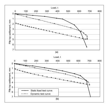
Fig 4 Load versus settlement for *(a)* pile no P359-1 *(b)* pile no P355-03 (Elevated structures on Kohat Enclave to Rithala)
