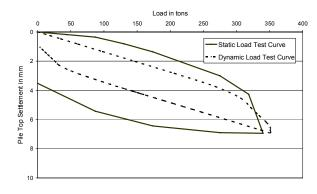
Fig. 5 Static Vs. PDA Test Match at Bangalore
