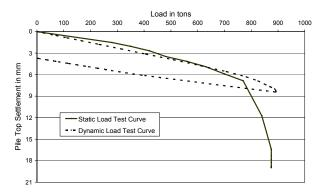
Fig. 4 Static Vs. PDA Test Match for TP3 at Chennai
