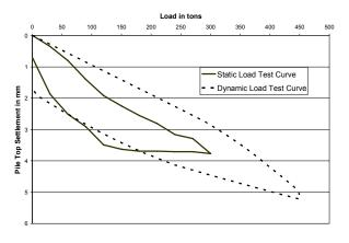
Fig. 6 Static Vs. PDA Test Match at Cochin
