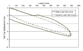
Fig. 3 Static Vs. PDA Test Match for TP2 at Chennai
