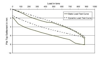
Fig. 2 Static Vs. PDA Test Match for TP1 at Chennai
