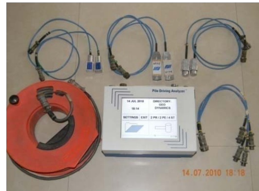
PDA Equipment and Sensors
