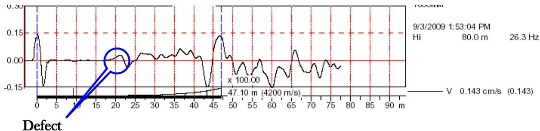
Figure 2 LSIT data indicating defect in the pile
