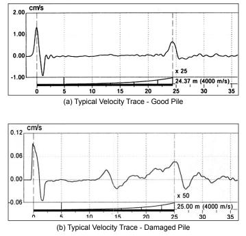
Figure 2 : Low Strain Integrity Testing by Pulse Echo Method
