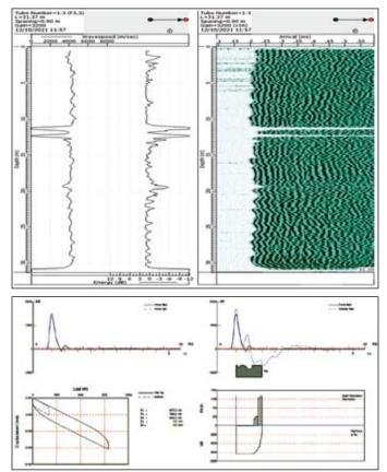
Figure 11 : CSL & HSDPT results on the same pile
