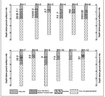
Figure 9 : Subsurface profile – A site in Mumbai
