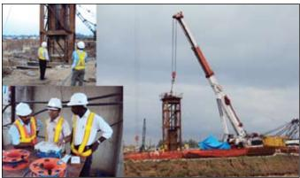
Figure 7 HSDPT in progress using 35 ton hammer
