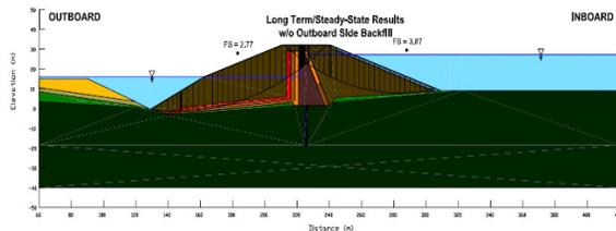
Fig. 5 Long Term Steady State Static Stability Analysis
