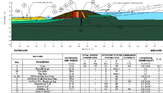
Fig. 3 Static Stability and Seepage Analysis – Typical Model
