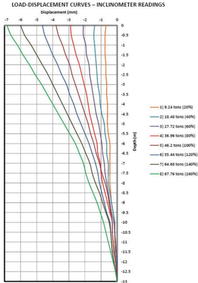
inferred that the pile undergone some deflection even at 12 m and below indicating that the actual point of fixity is somewhat lower than the theoretical calculations.
