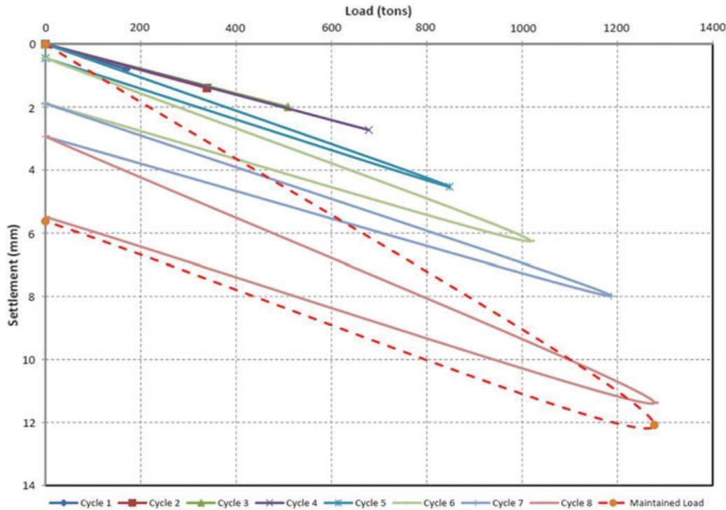
**Fig. 2** Load–settlement plot—vertical load test
