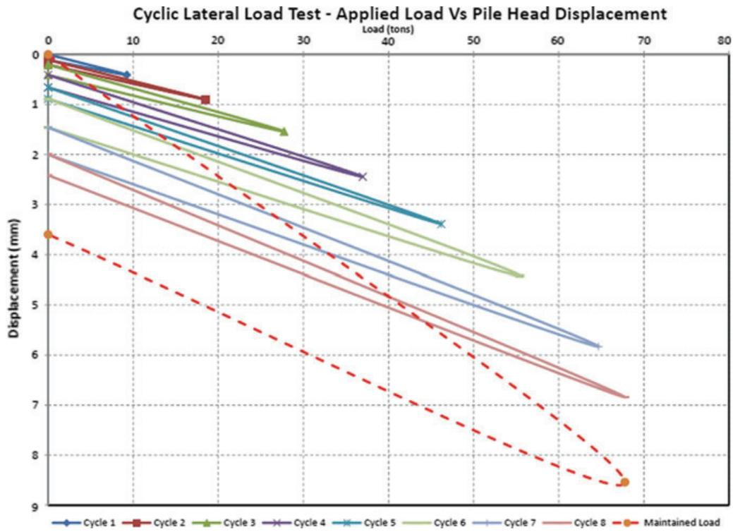
Fig. 6 Load–displacement plot—lateral load test
