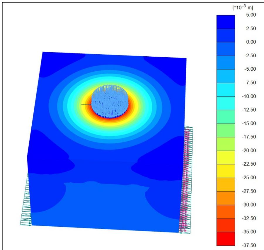
**Figure 8: Z-displacement contour (in m) obtained for seismic case in PLAXIS3D**
