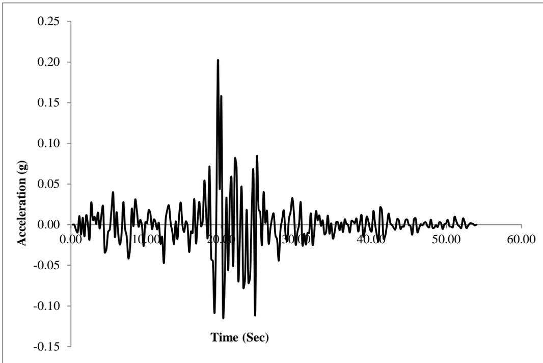
**Figure 9: Acceleration response obtained at the top of pile cap in PLAXIS3D**
