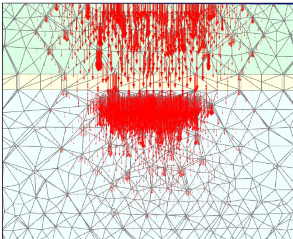
**Figure 6: Displacement vector diagram obtained for static case in PLAXIS3D**
