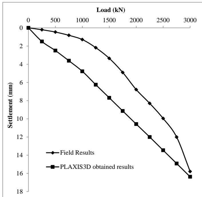
**Figure 3: Comparison of PLAXIS3D obtained results with field measured results**
