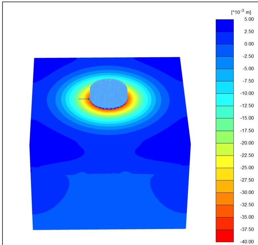
**Figure 5: Z-displacement contour (in m) obtained for static case in PLAXIS3D**
