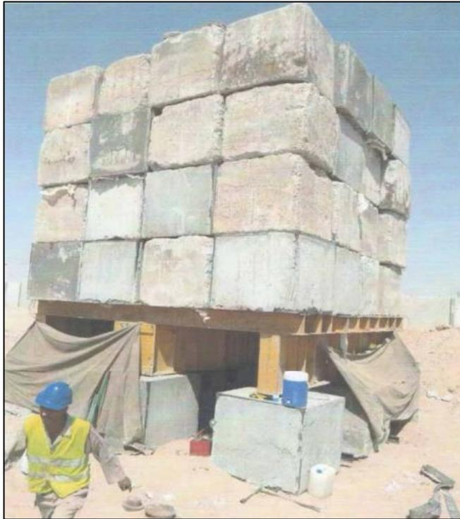
**Figure 2: Setup for Pile load test in Iraq**
