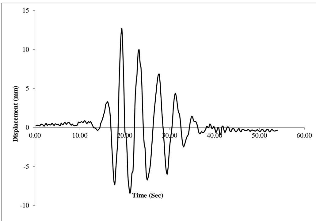
**Figure 10: Displacement response at the top of pile cap in PLAXIS3D**
