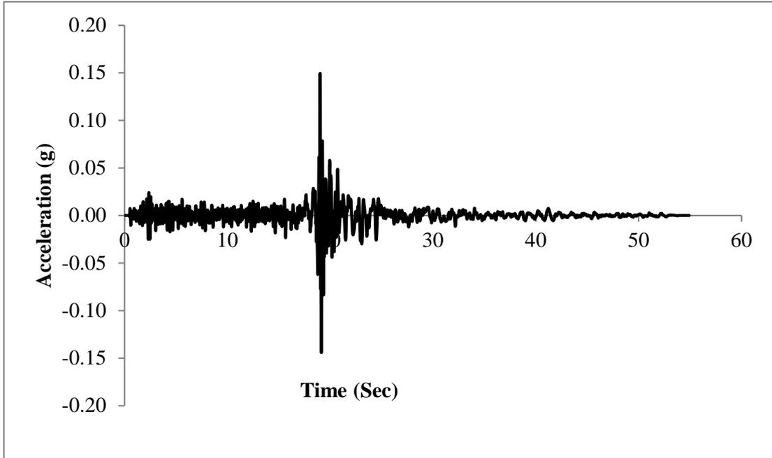
**Figure 7: Acceleration-time history used an Input in PLAXIS3D**
