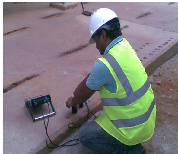
Fig. 2 Measurement of UPV tests on each specified grid.
