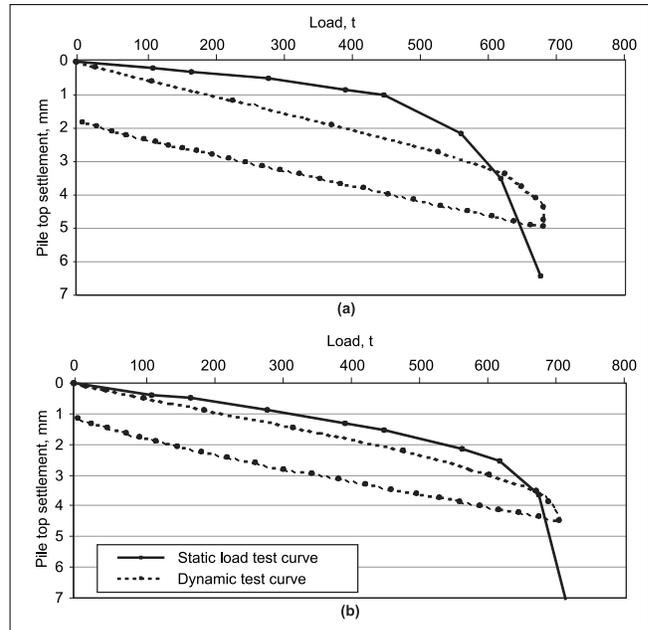
Fig 4 Load versus settlement for (a) pile no P359-1 (b) pile no P355-03 (Elevated structures on Kohat Enclave to Rithala)
