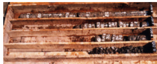
Figure 4. Photograph of the cores of pile A
