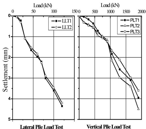
Fig. 7 Results of lateral and vertical pile load tests
