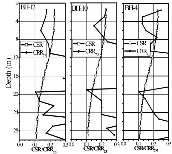
Fig. 4 Variation of CSR and  $CRR_{7.5}$  (based on SPT values) values with depth for some typical boreholes
