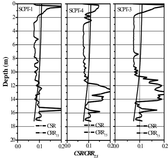
Fig. 5 Variation of CSR and  $CRR_{7.5}$  (based on CPT values) values with depth for different SCPT.
