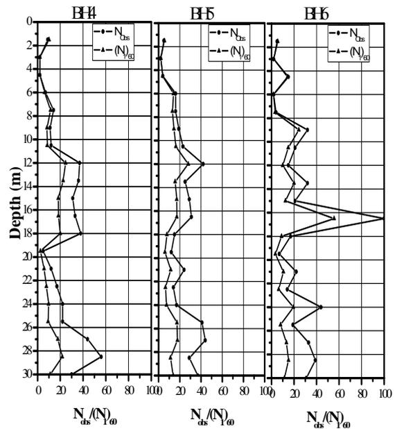
Fig. 2 Observed and corrected N-values at various depths for some typical boreholes
