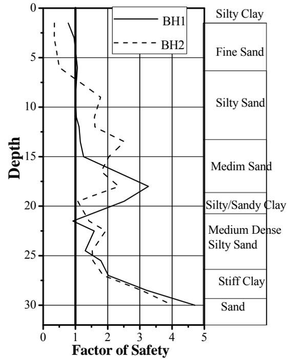
Fig. 6 Variation of factor of safety for some typical boreholes
