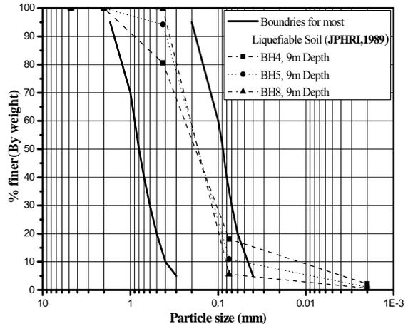
Fig. 3 Particle size distributions of samples for some typical boreholes
