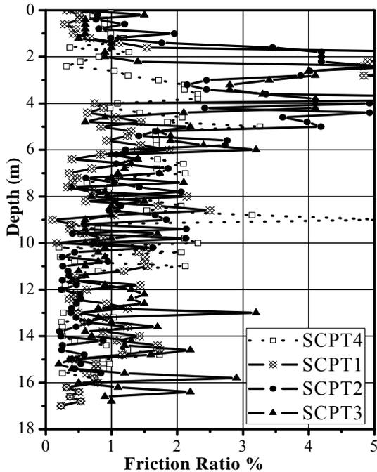
Fig. 1 Variation of depth vs. friction ratio (%) for different SCPT
